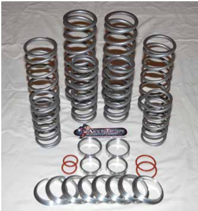
Here's the Stage 4 Fox Edition spring kit with silent cross-over collars and spring spacers. Front springs are 3.0 and rears are 3.75 inches. Individuals sell for $199 and $249, respectively.
