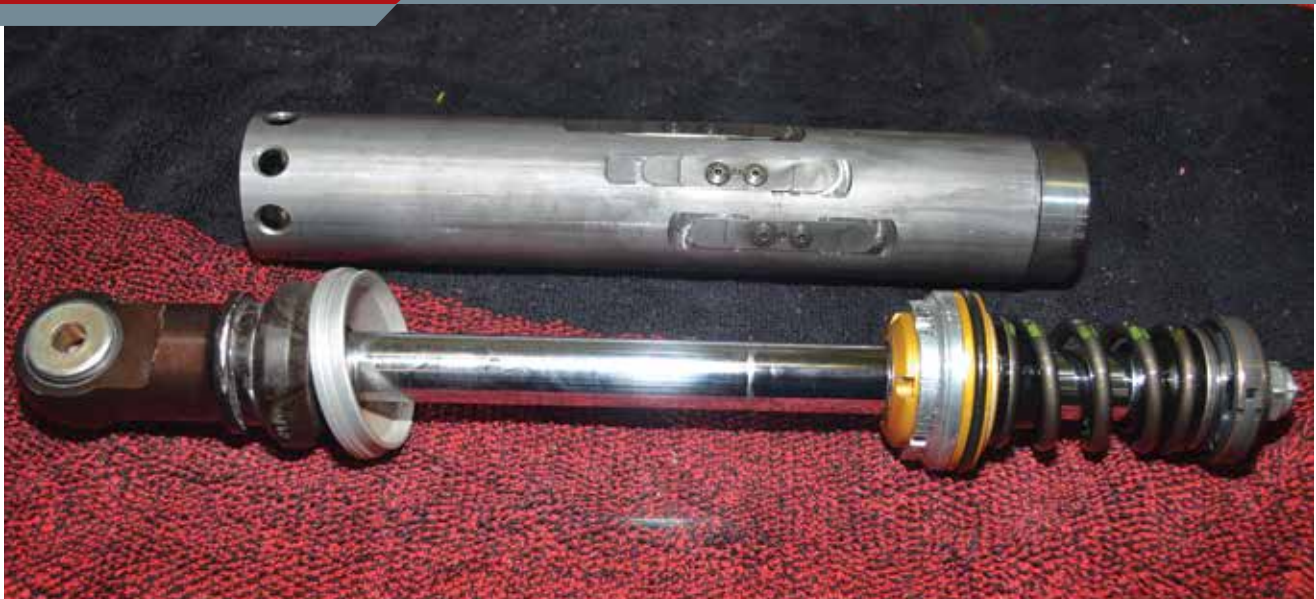
Here's the Fox Edition IBP sleeve with three offset reed valves and the shock-shaft assembly. Notice that the compression valve stack is backed up by a large spring that allows additional blow-off on big hits. ST stiffens the reeds, frees up the compression side of the piston, and lightens overall compression valving for plushness.
