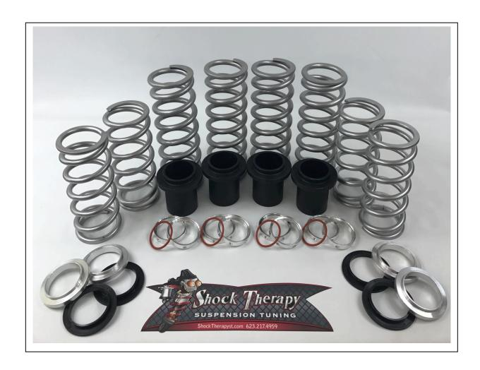
Thank you for purchasing our RZR General 4 seat 2015-2016 DRS kit. First, lay out your parts and springs, you should have 8 springs, 4 aluminum spring adaptor rings, 4 nylon spring adaptor rings, 4 nylon spring DIVIDERS and 8 silent cross over rings with 4 O-rings.
